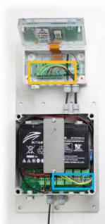
The inputs shown in the blue box connect directly to the inputs in the yellow box on the Metron4 above
